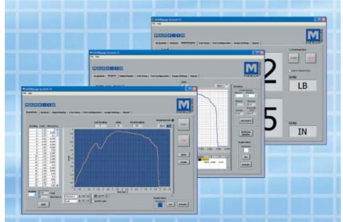
The program includes a set of tools to analyze test results, including statistical calculations, quick data export to Microsoft Excel, customizable reports, pass/fail indicators, and many others. Test setups and sequences are customizable and can be saved and recalled. The user can program test start and stop conditions, including load, time, distance, and sample break.
